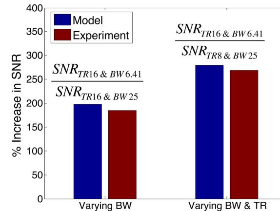
Fig 6: Percent increase in SNR by varying BW and/or TR, calculated from mid-volume circular ROI. 24 time phases were scanned at a TR of 8 ms and 12 time phases were scanned at a TR of 16 ms.
