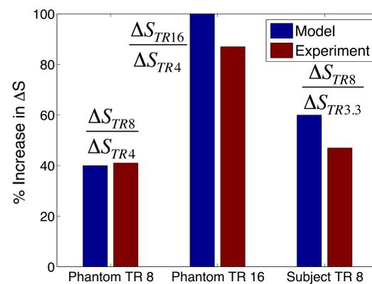
Fig 4: Comparison of the percent increase in  $\Delta S$  when longer TR is used compared to TR of 4 ms for phantom, and TR of 3.3 ms for patient. Model and experimental values are similar.
