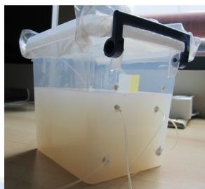
Fig 2: The phantom modeling brain tissue was made from dissolved agarose and Gd. Submerged PE and silicone tubing mimicked blood vessels. The phantom was scanned with saline and then with 8 mM Gd injected, at TR values of 4, 8, and 16 ms; other user-selected parameters were held constant.
