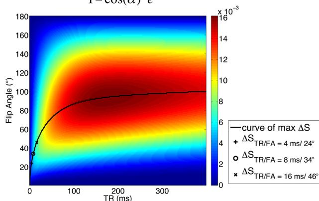
Fig 1:  $\Delta S(TR, \alpha)$  for WM using the SPGR equation. Constant parameters:  $TE = 1.4$  ms,  $T_1 = 1.1$  s,  $T_2^* = 70$  ms,  $r_1 = 3.3$  [Hz/mM],  $r_2 = 5.2$  [Hz/mM], [Gd in arterial blood] = 8 mM. The maximum  $\Delta S$  curve shows the optimal pairs of TR and  $\alpha$ .
