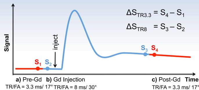
Fig 3: The sequence of scans acquired pre- and post-Gd injection.  $\Delta S$  is calculated by subtracting the baseline signal from the post Gd signal (rather than peak signal) for direct comparison between  $\Delta S_{TR3.3}$  and  $\Delta S_{TR8}$ . Assumption: there is no change in [Gd] between  $S_1$  &  $S_2$  and between  $S_3$  &  $S_4$ .
