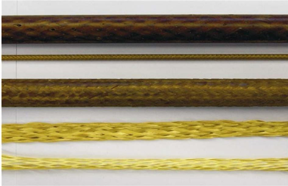
*Figure 6.1: Composite braids that are used in the manufacturing of catheters. These devices were made in a research lab and are not yet commercially available. Figure taken from ref (123).*
