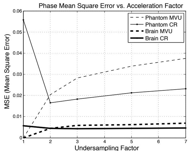
Fig 2: MSE vs Acceleration Factor. Data includes both phantom and *in vivo* measurements for a region measured inside the object.
